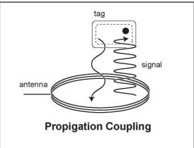
Tags and a reader communicate by wireless signal in a process known as coupling.
