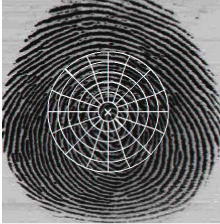
Figure 3.9: Reference point ( \times ), the region of interest, and 80 sectors ( B = 5, k = 16 ) superimposed on a fingerprint.
